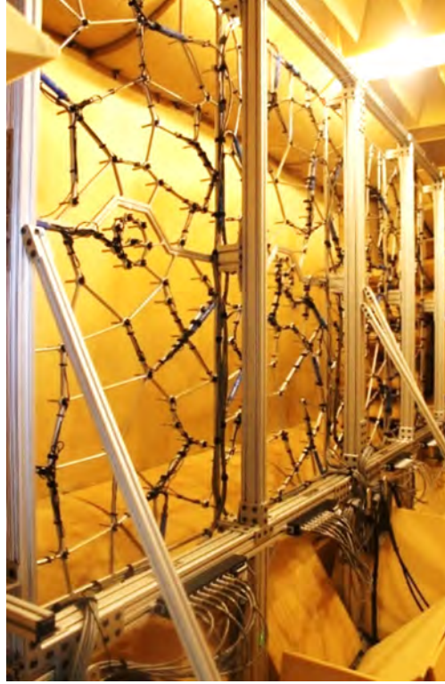
Fig. 5 AVEC 251-microphone array as seen from behind with a view of the starboard wall of the Stability Wind Tunnel Test Section
