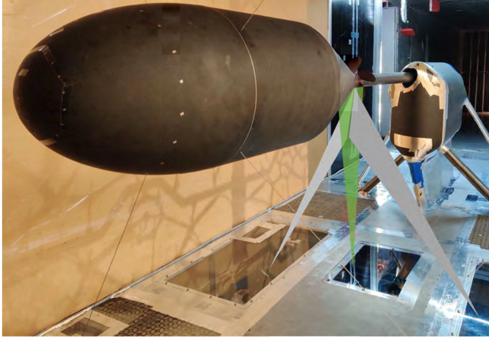
Fig. 7 Experimental photo showing the location of the PIV measurement plane and the laser and camera location setup for the 5° yaw starboard angle of attack configuration.
