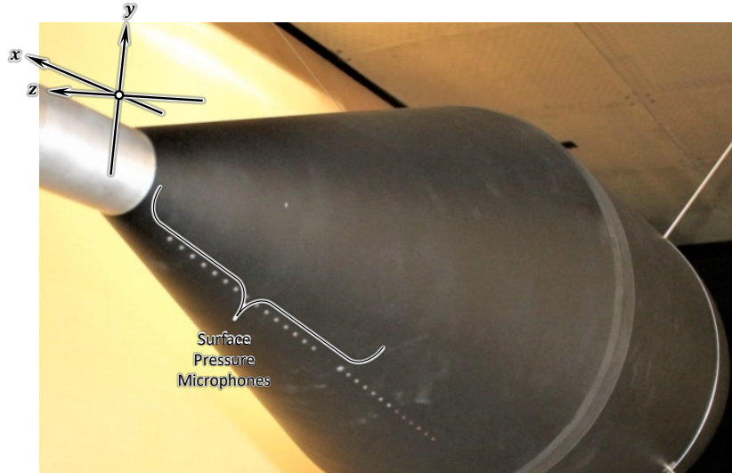
Fig. 4 Experimental photograph of streamwise array of flush-mounted Sennheiser microphones used to measure the unsteady surface pressure over the body of revolution tail cone
