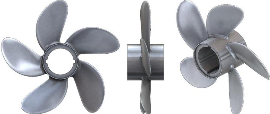
**Fig. 4: CAD of rotor wake-adapted to operate in the boundary layer of the body of revolution**
